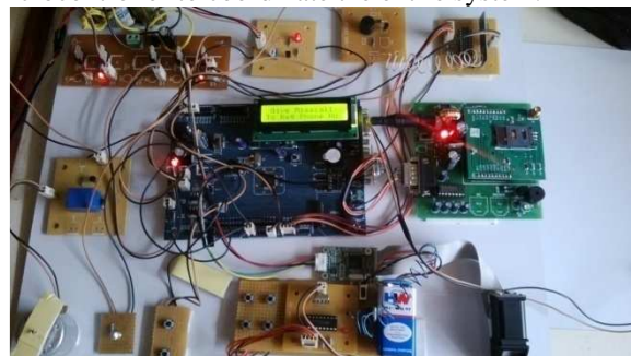
Fig 2: Multi level anti theft security system
